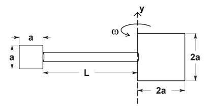
A wind vane consists of two vertical, light-metal, square slabs of equal density and equal thickness, and a thin rod connecting them. The squares have edge length a and 2a, respectively, and the thin rod has length L. The thickness of the squares and the diameter of the rod are negligibly small. The whole wind vane will rotate around the y-axis as the wind blows against it.
