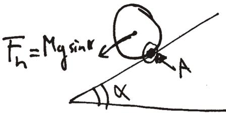
Determine torque + rotational inertia w.r. to the momentary stationary point A
