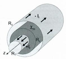
**4.a** Calculate the magnetic field **H** everywhere in space (i.e.  $0 < s < R_1$ ;  $R_1 < s < R_2$ ;  $R_2 < s < R_3$  and  $R_3 < s$ ). Give both the strengt *and* the direction of **H**.
