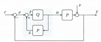
The gray box is the controller, and it contains a copy of the given system P. Notice that here  $\hat{r} = e + z$ .
