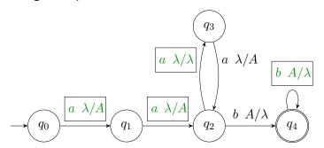
Complete the automaton such that it accepts L by filling the four white boxes. Note that we require this to be a deterministic, non-extended PDA. Only the symbol A may be pushed on the stack.
